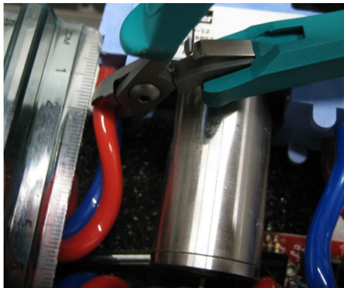
FIGURE H-10. Location of cuts to remove pump assembly from tubing
