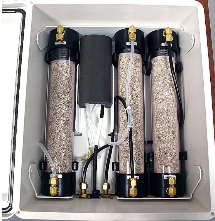
FIGURE G-3. Interior of CPEC200 scrub module with tubing and cover removed
