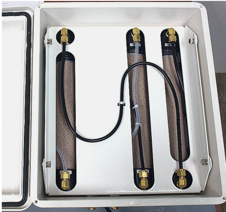
FIGURE G-2. Scrub module interior
